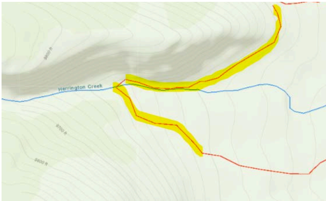
Figure 2. Examples of ditches running parallel to the grade.
