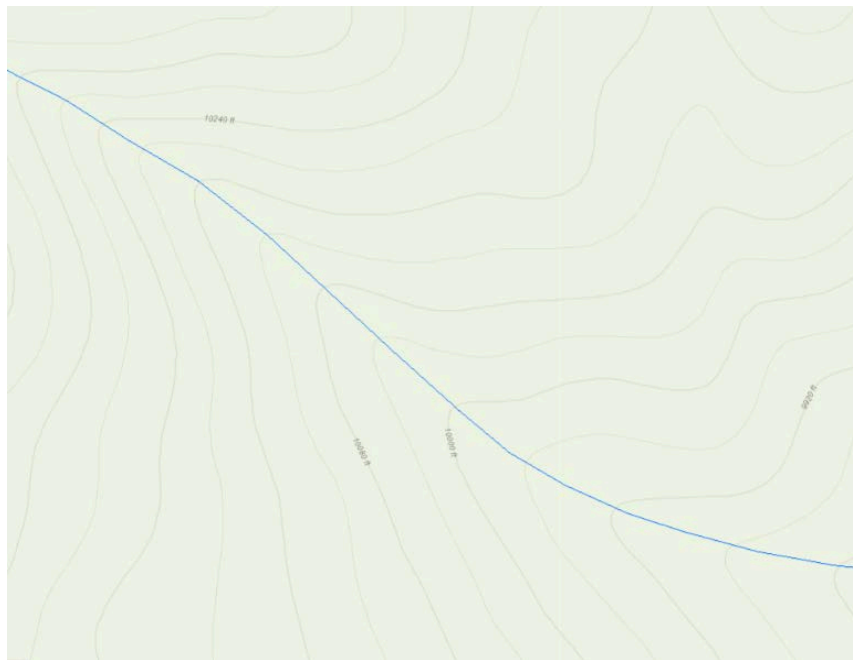
Figure 1. Example of a stream shown on topographic maps crossing the topographic lines, running perpendicular to the contour lines.
